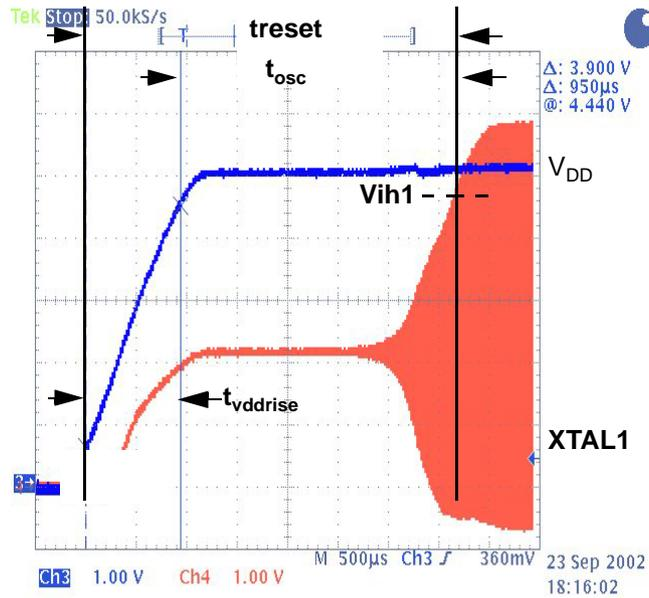
**Vih1** is the reference parameter taken to calculate and determine the time constant of the reset. Indeed, normally the input is considered to be low when its level reaches **Vil1**. But in reality the trigger is somewhere between **Vih1** and **Vil1**. So, the worst case condition is considered at the **Vih1** level.
