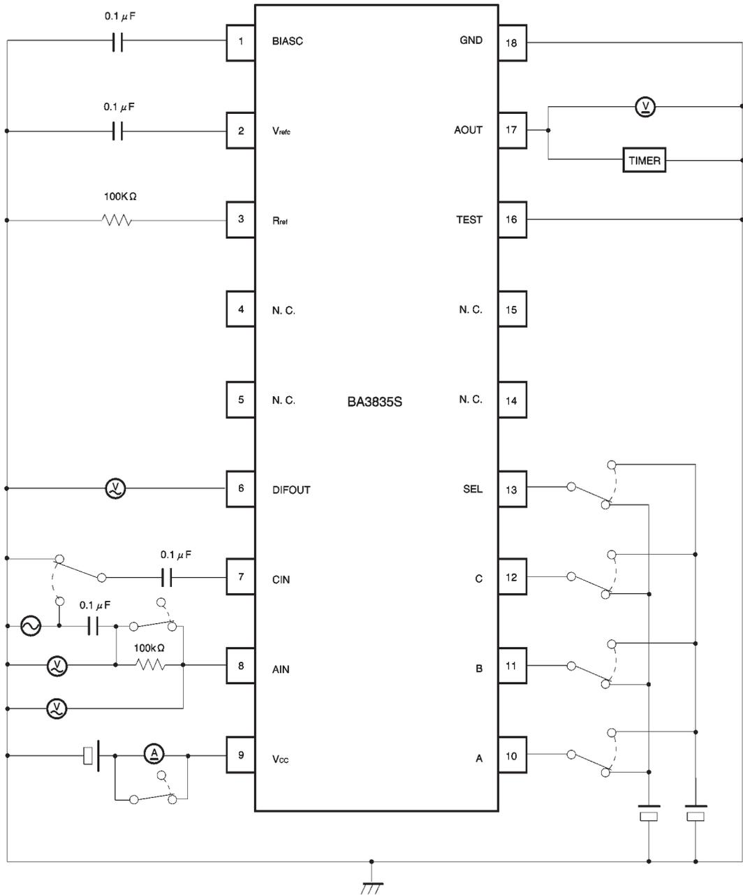
※The DIFOUT and SEL pins are different for the BA3835F.
