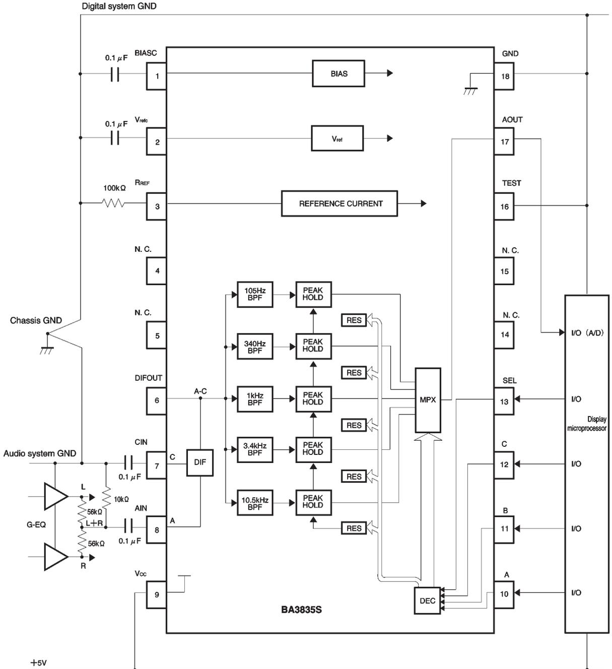
※ The DIFOUT and SEL pins are different for the BA3835F.
