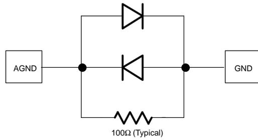
NOTE: GND and AGND must be tied to the same voltage level.
