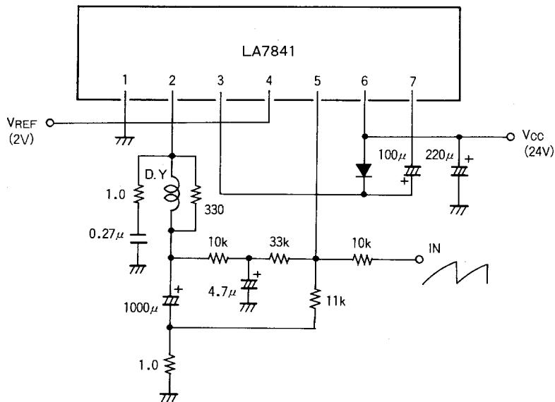
Unit (resistance: Ω, capacitance: F)
