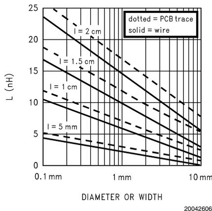
FIGURE 3. Inductance of Wire of Length 'l'
