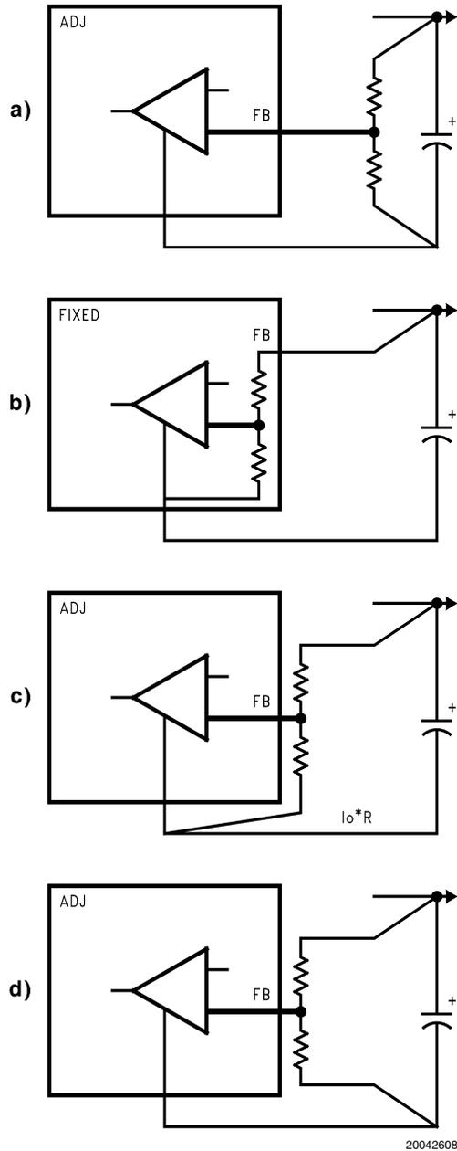
FIGURE 5. Feedback Traces (bold lines susceptible to noise)
