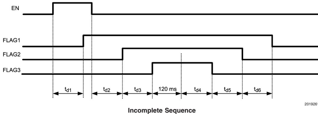
All the internal timers are generated by a master clock that has an extremely low tempco. This allows for tight accuracy across temperature and a consistent ratio between the individual timers. There is a slight additional delay of approximately 400us to timers 1 and 4 which is a result of the EPROM refresh. This refresh time is in addition to the programmed delay time and will be almost insignificant to all but the shortest of timer delays.
