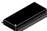
54 SOICW-EP 0.65 mm Pitch 17.9 mm x 7.5 mm Body 4.6 mm x 4.6 mm Exposed Pad
