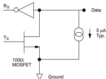
**BUS MASTER CIRCUIT** Figure 3**A) Open Drain**
