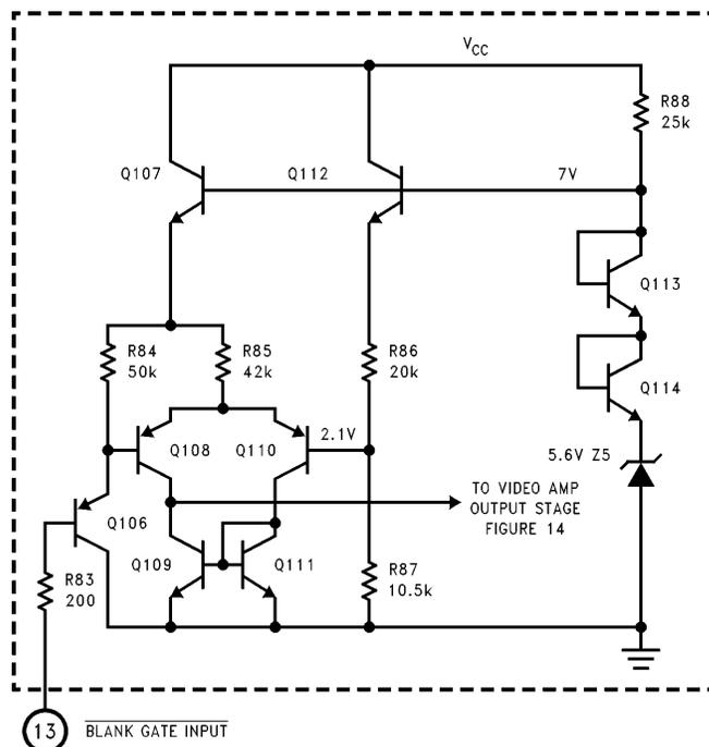
FIGURE 13. Simplified Schematic of LM1205 Blank Gate Circuit
